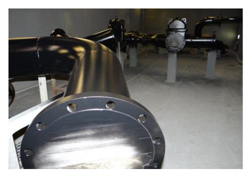
Rilmac Fabrication completed the fabrication and supply of two sets of fan casings with associated duct work. The units were successfully trial assembled in the workshop prior to installation at Tata Steel, Scunthorpe.
