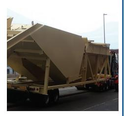
The larger Rustler 12 is over 8m x 17m x 3.5m and each one is completed on a trailer chassis, also made by Rilmac Fabrication, with the tractor unit able to drive each one from Rilmac's main workshop. Constructed from mild steel the Rustler 12 is a self-erecting remote batch plant designed to work with most ready mix, aggregate and cement options.
